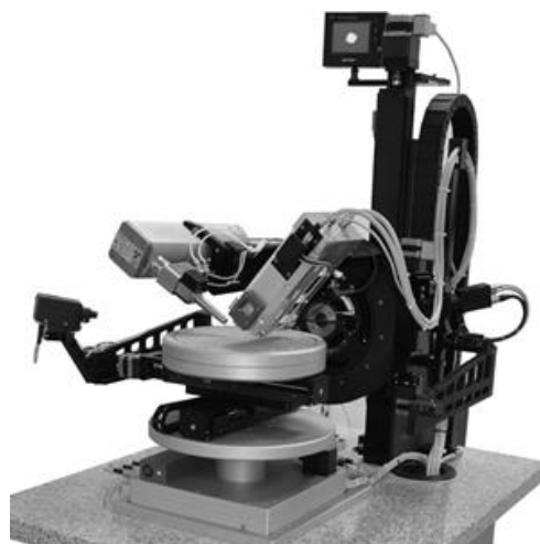
FIGURE 4. Diffractometer for combined Omega- and Theta-scan measurements; with arrangement for local mapping.
